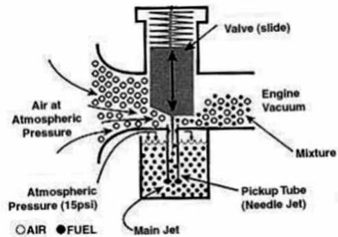
Both the CV and conventional slide carburettors, like Amals, are classified as variable venturi carbs. The slide on a conventional carburettor is directly connected to the throttle cable. Twist the throttle grip and the slide is raised in the venturi.
