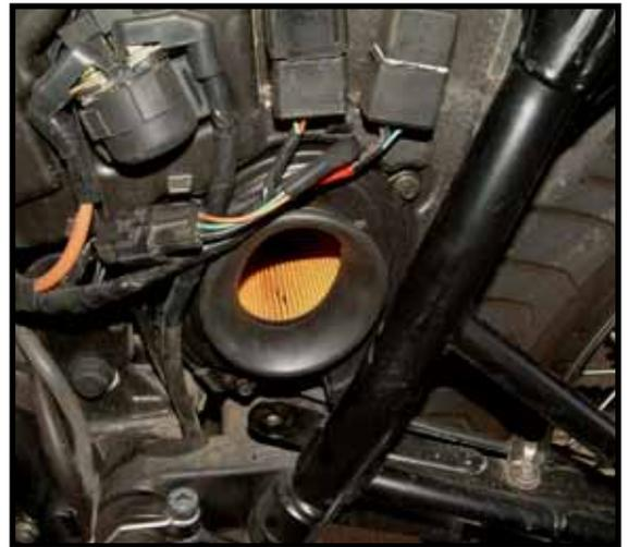
Fitted to a standard air box
