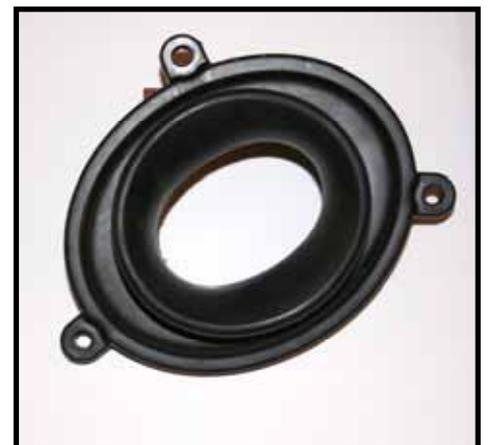
5. Fit the modified cover plate back to the airbox, tighten the screws to 3Nm and don't forget the small wire retaining clip. The picture below right shows the result with a modified airbox cover on an airbox removed from the bike. The rubber part has taken up an almost perfect shape.
